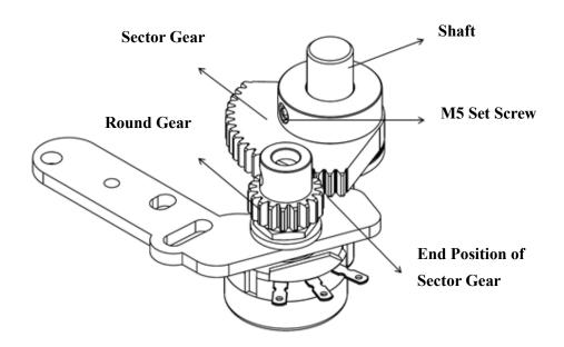
TC2 is utilized for sensing fully-closed stop point. Once the spring mechanism has been released when power outage, the actuator will not drive under power again until it has reached its fail stop position and TC2 trips.
