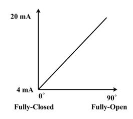
• When a high signal value received, the actuator operates toward fully-open position and when a low signal value received, the actuator operates toward fully-closed position.
