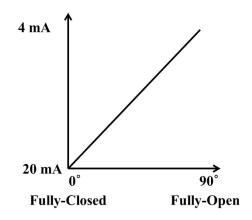
• When a low signal value is received, the actuator operates toward fully-open position and when a high signal value is received, the actuator operates toward fully-closed position.
